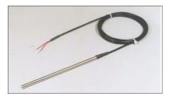
A general purpose Pt100, 3-wire sensor with a class B tolerance detector housed in a 316 stainless steel sheath 6 mm diameter x 150 mm long. Supplied with 2 m PTFE screened lead. Maximum temperature 250°C.
