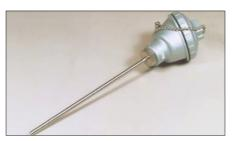
This industrial 4-wire Pt100 has a useful rating of 400°C. The class B sensor is housed in a 316 stainless steel sheath 6 mm diameter x 200 mm long mounted below our proven CE aluminium alloy terminal head rated IP65.
