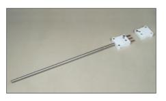
Intended as a low cost alternative to sensors with terminal heads, this Pt100 is terminated in a simple plug. The Class B, 3 wire sensor is housed in a 316 stainless steel sheath 3/16" diameter x 200 mm long. Supplied with mating socket for connection to your cable. Maximum temperature 250°C.
