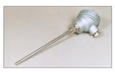
A similar sensor to 350-110, this 3-wire Class B Pt100 is housed in a 316 stainless steel sheath 6 mm diameter x 150 mm below a miniature KS aluminium alloy terminal head rated IP65 complete with ceramic terminal block.
