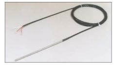
This fast response Pt100 has a specially designed construction to give better performance. The class A, 4-wire sensor is housed in a 316 stainless steel sheath 4 mm diameter x 150 mm long. Supplied with 2 m PTFE screened lead. Maximum temperature 200°C.
