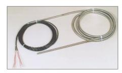
Our autoclave chamber probe has been designed in collaboration with leading autoclave manufacturers. The duplex, class A Pt100 is housed in a 6 mm dia x 200 mm long sheath with 2 m armoured lead, an entry tube 6 mm dia x 150 mm long and 3 m Silicone Rubber lead.
