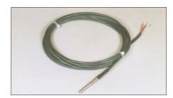
This sensor has a useful operating range but is also extremely low cost. The 3-wire, Class B Pt100 is housed in a 316 stainless steel sheath 4.8 mm diameter x 50 mm long and is supplied with 3 m silicone rubber lead. Maximum temperature 200°C.
